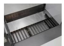
The EC-400/500 Series machines feature a wide belt-type chip conveyor positioned in the center of the machine, directly under the spindle, for vastly improved chip management. The steep walls of the interior enclosure easily funnel chips to the conveyor.
