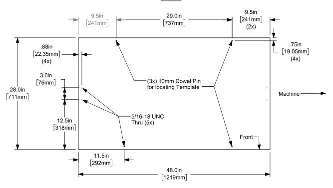
To accommodate the large variation in size and shape of material that can be loaded by the APL, use the following guidelines and table dimensions to make your own part specific templates
