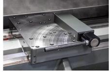
Fully Programmable Servo-Driven Tailstock - can be activated via the part program, or controlled directly with the standard foot switch. Features an MT5 or MT6 taper, depending on model, and provides up to 4500 lb of thrust.
