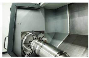
Extended Tool Pocket; provides clearance for long drills or boring bars when the turret is closest to the chuck.
